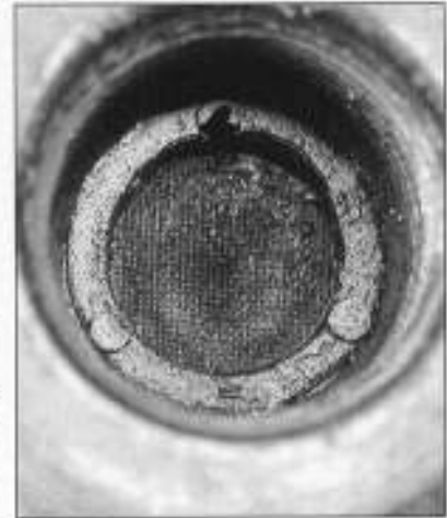
Corrosion clogging this inlet filter (right) and valve (top) might be circulating through the system, but corrosion also is occurring locally on the valve body housing and on the plunger inside (above).
