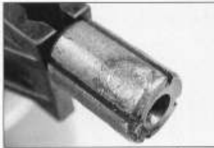
Corrosion clogging this inlet filter (right) and valve (top) might be circulating through the system, but corrosion also is occurring locally on the valve body housing and on the plunger inside (above).
