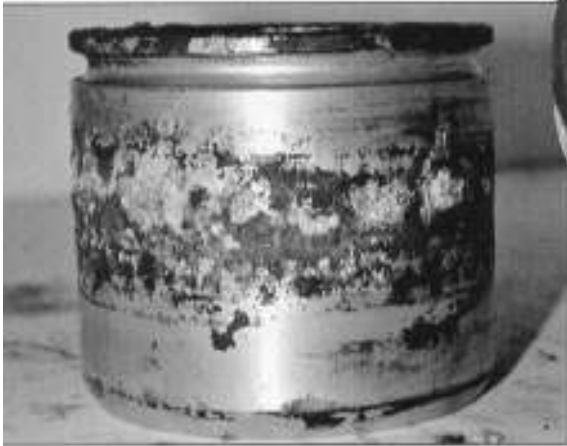
The corrosion on this caliper piston is mostly likely caused by environmental conditions. When circulated by ABS operation, deposits can be transported to other parts in the system.
