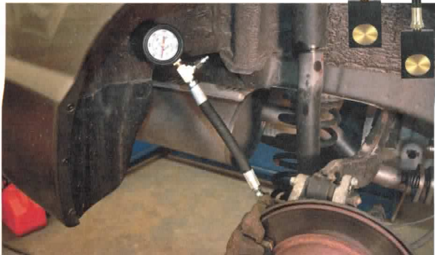
The Hickok/Waekon gauge from the Hydraulic Pressure Test Kit connects to the rear calipers of a 2006 Honda Civic. For information about this product, go to www.VehicleServicePros.com/10772314 .
