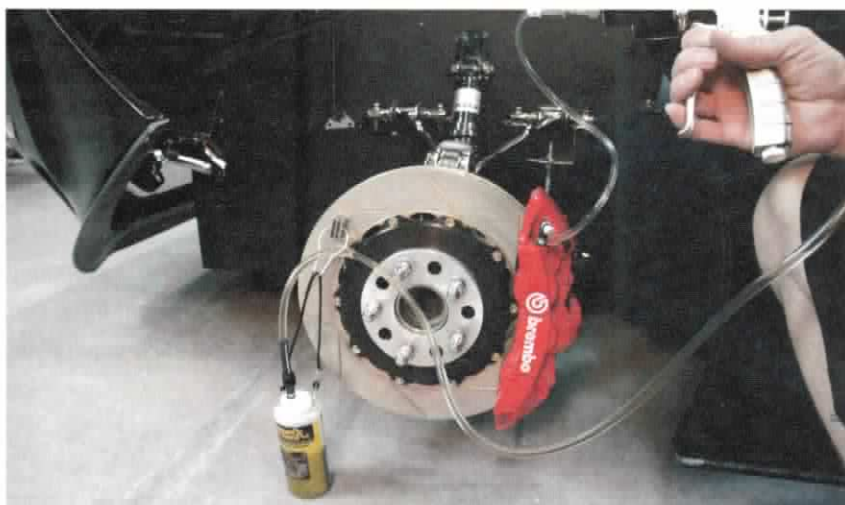
Phoenix Systems' MaxPro Brake Bleeder, with the help of different adapters, can pressure, vacuum and reverse bleed a vehicle. For information on this product, go to www.VehicleServicePros.com/10721444 .
