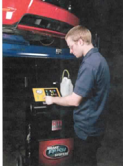
RTI's BFX-2 Brake Fluid Exchange System pushes fluid through the master cylinder, while simultaneously applying vacuum to the appropriate bleeder. For information on this product, go to www.VehicleServicePros.com/10099737 .
