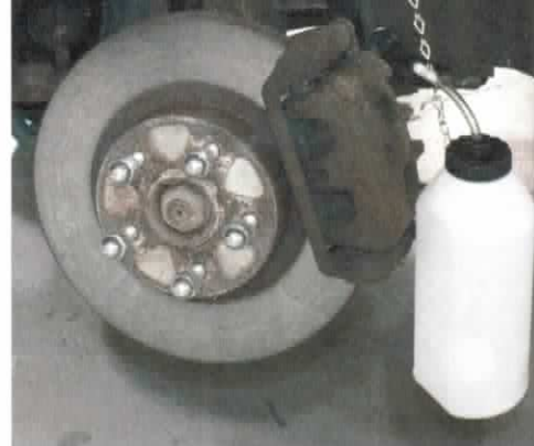
The BrakeMate Jr. from Flo-Dynamics eliminates suction lines and includes a catch bottle giving the tech the freedom to follow the bleeding sequence himself. For information on this product, go to www.VehicleServicePros.com/10106064 .
