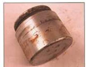
Fig. 2: Minor corrosion of a caliper piston
