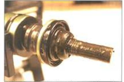
Fig. 5: The sludge buildup in the unused bore of the master cylinder can cause primary cup seal damage if the brake pedal is depressed too far.
