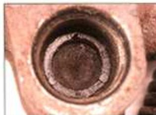
Fig. 8: This is the inlet filter to a RWAL/RABS valve. Notice the restriction starting in the top portion of the filter screen. I have seen these filters restrict to a point where there is little to no braking in the rears and also restrict the fluid flow back to the master cylinder. Every modulator I have ever disassembled has multiple filters. Due to corrosion, some of these filters are prone to plugging.
