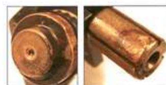
Fig. 11 & 12: Kelsey Hayes ABS systems use dump valves and low pressure accumulators in their modulators. The dump valve seat can corrode to a point where fluid is allowed into the low pressure accumulator during normal braking. See the related article for more detail. By-passing dump valves is a common problem on these systems and was noted in the NHTSA report referenced by force.
