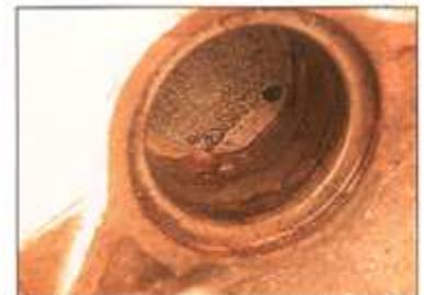
Fig. 1: Internal corrosion of caliper bore. Those of us that have been around long enough to have rebuilt calipers, recognize this picture. The brake fluid in the calipers is typically the worst in the system. This is due to the reason given above, plus the fact that they are the lowest point in the system.
