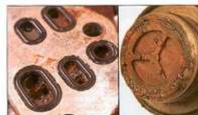
Fig. 13 & 14: These figures show the internals of a TEVES 4 ABS system. This modulator is mounted low on the vehicle so it suffers some of the same problems as the calipers. Figure 13 shows the modulator body passages and it is easy to see the amount of corrosion that has taken place. Figure 14 shows one of the isolation valves and it is clear that the filter is being affected by the corrosion that has taken place.
