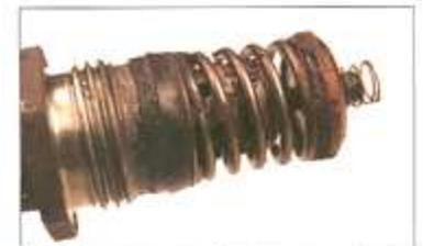
Fig. 6: Corrosion can affect the conventional valving of a vehicle, as seen on the internals of this metering valve. As can be seen from the image, the amount of buildup is significant.
