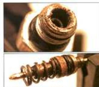
Fig. 9 & 10: Certain early Kelsey Hayes ABS rear-wheel and four-wheel ABS systems use reset switches to signal the end of an ABS cycle. The reset switch cap and piston for an EBC2 system are shown in Figures 9 & 10. Code 4, the result of a grounded reset switch, is one of the most common failures in this type of system. The reset switch return spring can't push the piston back to a rest position.
