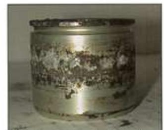
Fig. 3: Severe corrosion of the caliper piston.
